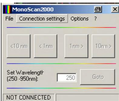
7. Go to the Connection settings menu and select the Comport to which the MonoScan-2000 is connected.
